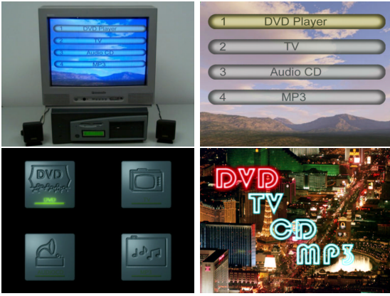
Figure 2: The Multimedia-Box and the main menu rendered in different styles or skins .
